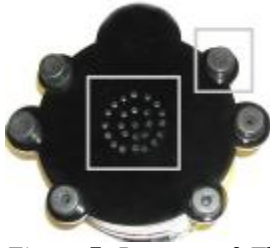
Figure 7. Prototype 2, The bottom view of the toy shows its supporting legs and the openings for the sound coming from the speaker
