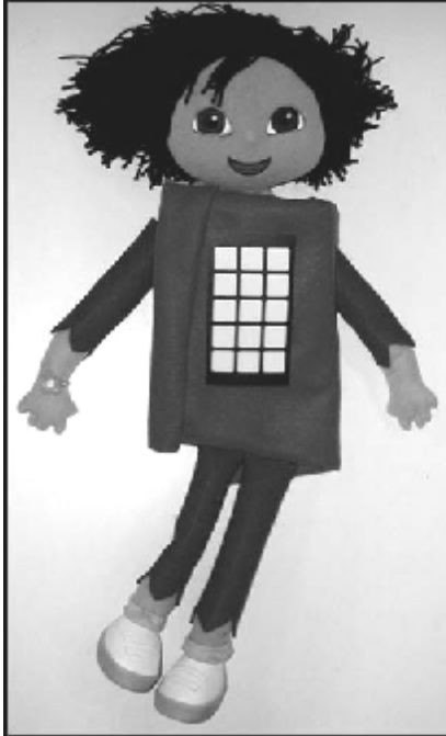
Figure 1. Prototype 1: The Doll Mary-Marie has a button interface which reads the tags on her different dresses and tells a story in French and English.
