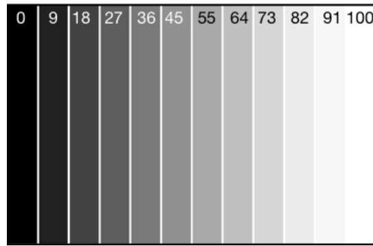
Figure 3.1: Each roll of film was exposed to this image. The first rectangle, labeled '0', is 0% grayscale, or black. The left most rectangle is 100% grayscale, white. The full image represents the full grayscale spectrum is labeled by percent grayscale. Strips were chosen for ease of analysis and the full spectrum was represented to explore if the amount of light or shadow in an image affects the amount of reticulation.
